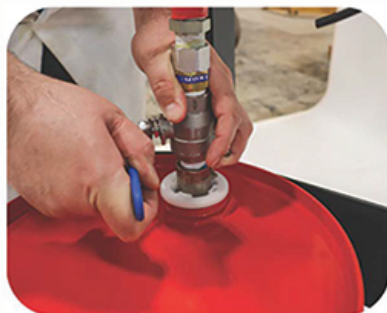
Twist Lock Hose Connection (inserted in drum bung)
