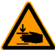
Risk of crushing
