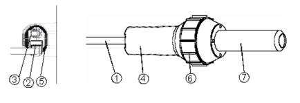
1Power supply cord5Air filter2Main switch6Rubber stand3Potentiometer for temperature adjustment7Heater tube4Handle7Heater tube
