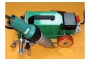
Simple to operate and very reliable because of robust design. Available for 20, 30 or 40 mm width welding seam.
